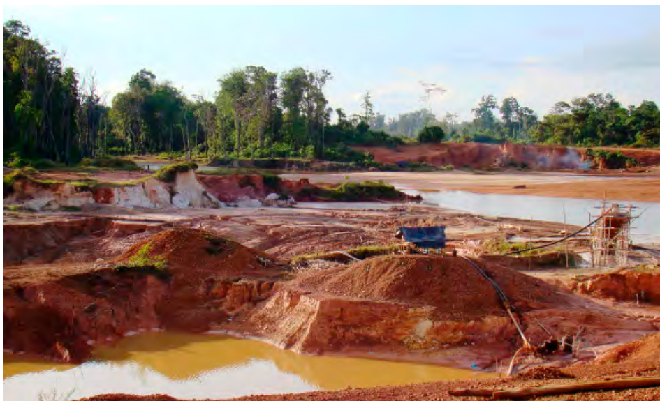
FIGURE 7 Destruction produced by hydraulic monitors mining, an example at Las Claritas mine
